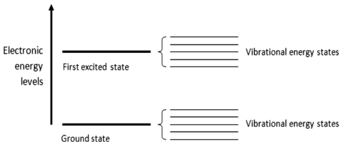
Fig. 10.1. A schematic representation of the quantized electronic and vibrational energy levels of a molecule: to raise the electronic energy state of a molecule from the ground state to the excited state will cost more energy than to raise the vibrational energy state
